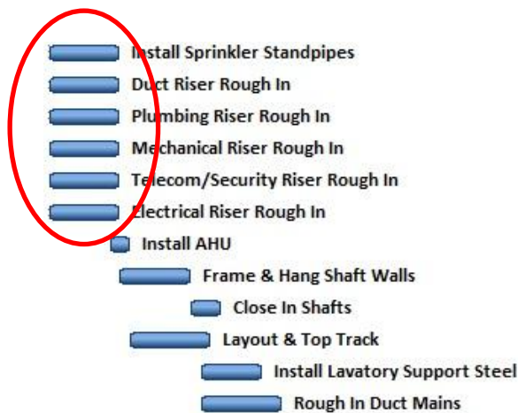
Figure 26: All riser activities occur simultaneously, so even if electrical riser finishes, the following activities cannot start until the remaining riser work is complete.
